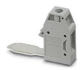
Pick-off terminal block, Connection method: Screw connection, Cross section: 0.5 mm² - 10 mm², AWG: 20 - 8, Width: 10.2 mm, Height: 34.7 mm, Color: gray, Mounting type: On base element
